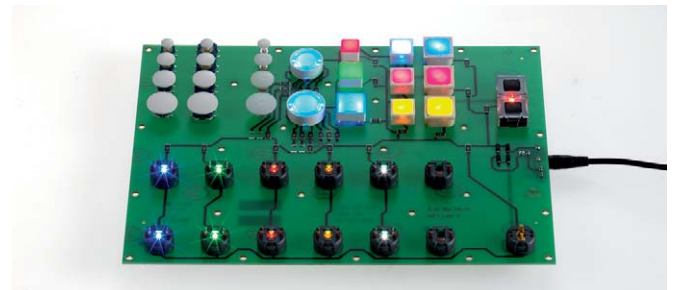
Top half: RAFI short-travel keyswitches RACON 8/12, MICON 5, RF 15/19, short-travel mains switch KN 19 Bottom half: RAFIX FS contact blocks, some with 3 mm THT LEDs
