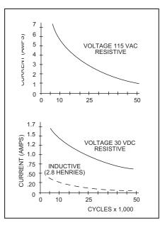
These curves allow you to predict the expected life of the switch once you know the voltage, current and type of load. Also note that each cycle is approximately a 360° rotation and a return. For a ten position switch this would be a rotation from position 1 to position 10 and back to 1. This cycle runs approximately ten times a minute. Thus testing causes more electrical and mechanical wear than what the switch incurs in actual use.
