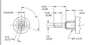
Metric standard dimensions for the shaft and bushing are shown in the drawing. Other dimensions approximately the same as shown in dimensional drawing. Contact Grayhill for exact dimensions. See Style "E" in the Choices and Limitations chart.
