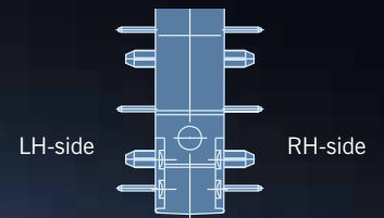
Side definition with terminals and location pins
