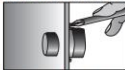
The holder will be secured at the back by two screws or nut.
