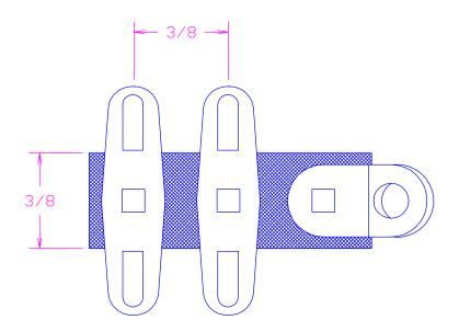
LUG: PLATED STEEL, SPACED 3/8" CENTER STRIP: XP PHENOLIC 3/8" WIDE x .062"THICK.
