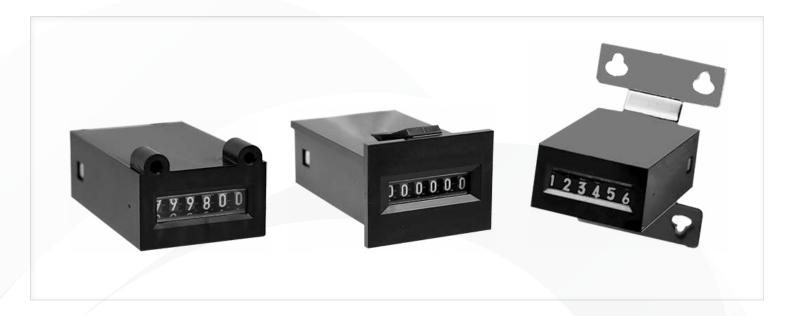
A 6 figure, non-reset counter. Metal/plastic frame assembly assures ruggedness while one piece cover discourages tampering. Precision molded internal gearing requires no lubrication for long, accurate count life. Applications include warranty verification, electronic game counting, coin box tallies, or wherever small size, highly visible numerals, and solid construction are critical.
