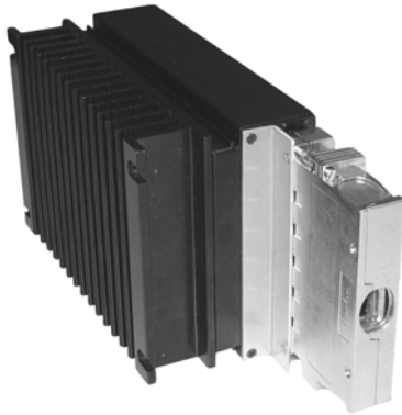
Fig. 47 Different cable hoods
