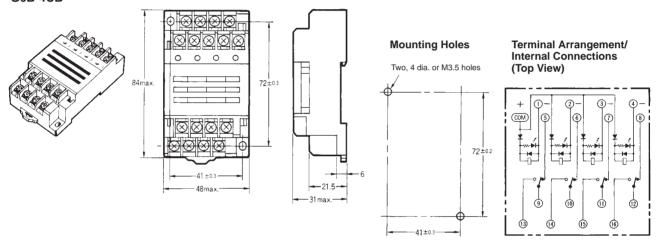
Note: Do not reverse the coil polarity.
